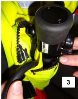
Continue feeding the hose into the inner pocket (Figure 3). Until the majority of the hose is positioned inside the pocket (Figure 4)
