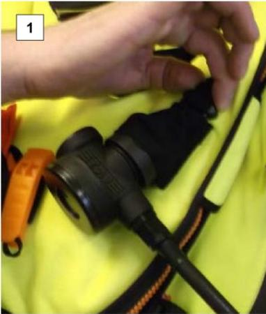
The Heliport Suit Technician will remove the HUEBA mouthpiece retainer (with mouthpiece attached) from the LPU by means of releasing the clip (Figure 1), then open the HUEBA pocket zipper and remove the HUEBA from the pocket (Figure 2) and place it into the HUEBA carrying bin (to prevent damage)
