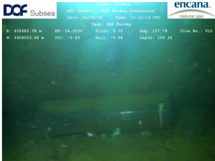
Soft debris (plastic) at KP 54.055
