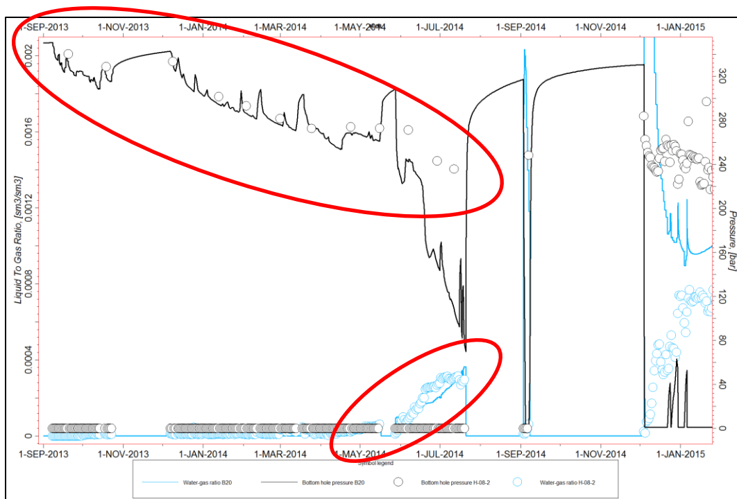
Figure 5.5.1.3: Panuke H-08 history match. The pressure and WGR matches were reasonable before water production from the well started. Match quality was lower after the start of water production.
