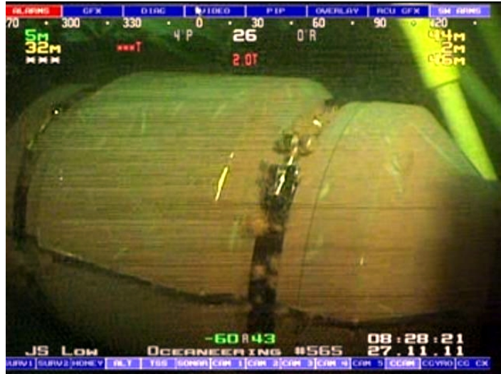
Tubularian hydroids sparsely colonizing straps of insulation cover of flowline M-79A in 2011 the survey
