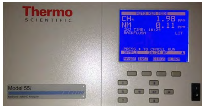
Figure 33. 55i Thermo Scientific Methane and Total Non-methane Hydrocarbon (VOC) Analyser
