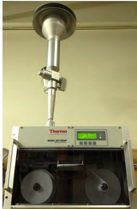
Figure 32. Thermo Model 5012 Multi-Angle Absorption Photometer (MAAP) black carbon analyzer
