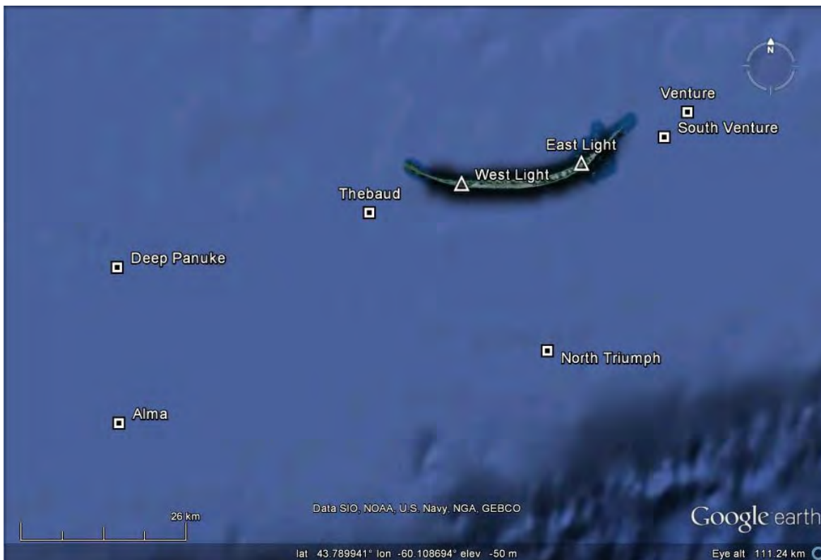
Figure 4.1-2 – Location of offshore natural gas platforms surrounding Sable Island (43.93°N, 59.90°W, approximate centre). Sable Island is approximately 40 km in length, and 1.2 km wide at the centre. Receiver stations were deployed at West Light and East Light on Sable Island. In 2013, additional receivers stations were deployed with 1 km of each of the tips of the island.
