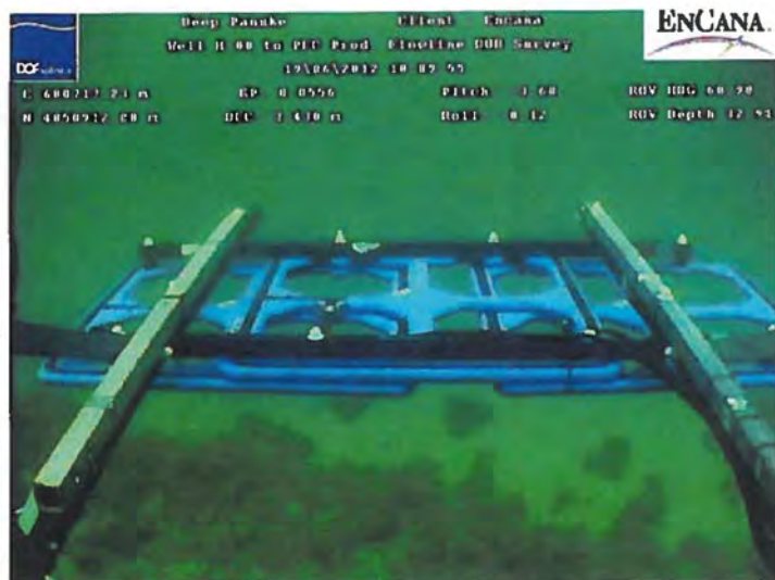
End of rock dump and buried flowline to wellhead H-08 with sandy seafloor and large patches of the sea cucumber Cucumaria frondosa
